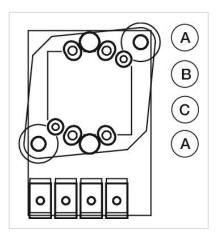
A = 4 = Switch B = x+ = LED Anode (+) C = 1x- = LED Cathode (-)
