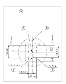
A = Drilling plan (component side)
