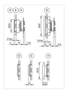
A = Lens level with bezel E = Lens raised above bezel H = Mushroom-head cap
