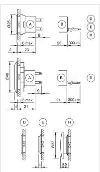
A = Plug-in terminal 2.8 mm x 0.8 mm B = Flat ribbon cable
