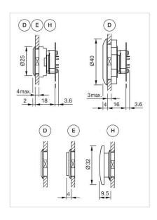
A = Lens level with bezel E = Lens raised above bezel
