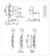
A = Plug-in terminal 2.8 mm x 0.8 mm B = Flat ribbon cable D = Lens level with bezel
