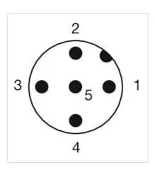
1 = NC 2 = LED+ 3 = Common 4 = LED-5 = NO A-Coded
