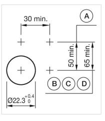
A = Screw terminal B = Push-in terminal (PIT) C = Plug-in terminal 6.3 mm x 0.8 mm D = Double plug-in terminal 6.3 mm x 0.8 mm
