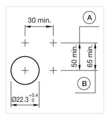
A = Screw terminal B = Push-in terminal (PIT)
