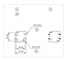
A = Switching element with illumination B = Single LED C = Drilling plan (component side) D = Hole for switching
