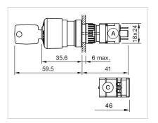
A = Plug-in terminal 2.8 mm x 0.5 mm C = Screw terminal
