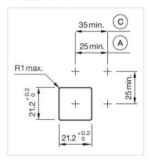
A = Solder/Plug-in terminal 2.8 mm x 0.5 mm C = Screw terminal
