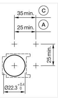
A = Solder/Plug-in terminal 2.8 mm x 0.5 mm C = Screw terminal
