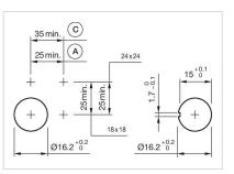
A = Solder/Plug-in terminal 2.8 mm x 0.5 mm C = Screw terminal
