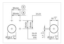
A = Solder/Plug-in terminal 2.8 mm x 0.5 mm C = Screw terminal
