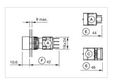
A = Plug-in terminal 2.8 mm x 0.5 mm C = Screw terminal E = Slow-make switching element F = Snap-action switching element
