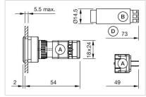
A = Plug-in terminal 2.8 mm x 0.5 mm B = Solder terminal
