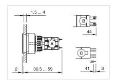
A = Solder terminal B = Plug-in terminal 2.8 mm x 0.5 mm C = Universal terminal 2.0 mm x 0.5 mm
