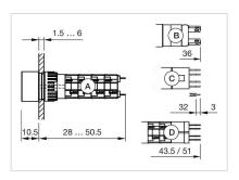
A = Solder terminal B = Plug-in terminal 2.8 mm x 0.5 mm
