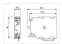
B = Spring-type terminal for Part No. 45-317.1Z40
