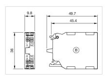
B = Spring-type terminal for Part No. 45-316.1X40
