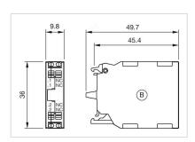
B = Spring-type terminal for Part No. 45-314.1X40
