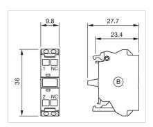
B = Spring-type terminal for Part No. 45-312.1Z40, 45-312.1X40
