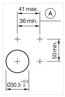
A = Action range of aligning pins
