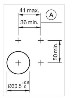
A = Action range of aligning pins
