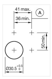
A = Action range of aligning pins
