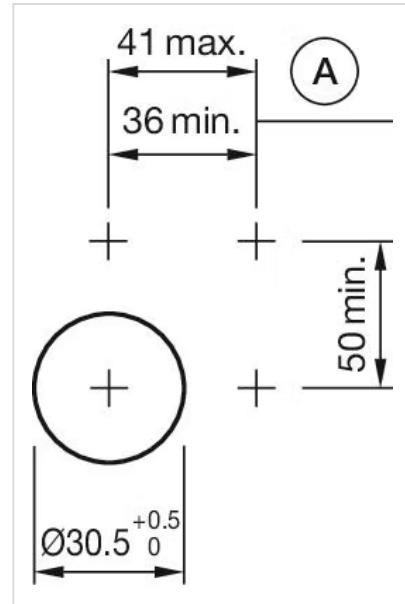
A = Action range of aligning pins
