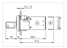
A = Screw terminal B = Plug-in terminal 6.3 mm x 0.8 mm
