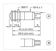
A = Protection tube (only 230 VAC) B = Tri-colour
